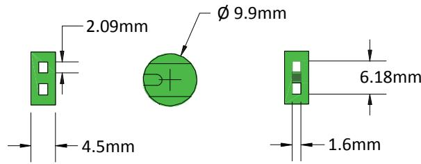
The YP10 Seal is manufactured from ABS material and is suitable for applications where the traditional lead seals cannot be used. Effective closure is achieved with the DMC sealing tool LP2.
